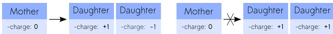
Figure 58: Example for a basic decay, here for the electric charge quantum number. When charge conservation is active the right charge decay example is forbidden and will be retracted by the expert system charge conservation rule.
