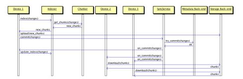
Fig. 1. Interaction between the components of sync engine for a Personal Cloud.
