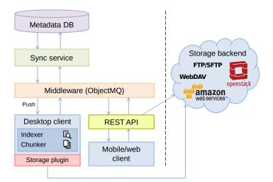
Fig. 2. StackSync architecture
