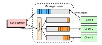
Fig. 3. Message broker communication flow
